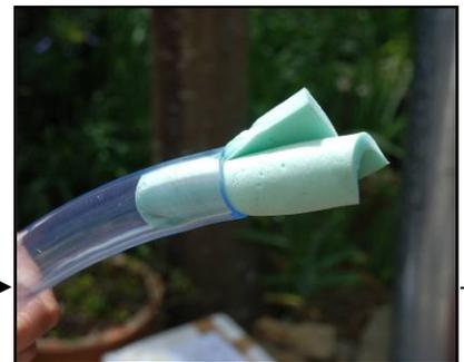
**3)** Block up the open end with a watertight seal and hold the funnel end vertical so the water stays contained in the tube.
