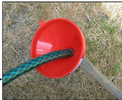
**2)** Fill the tube with water from a garden hose, making sure there are no air spaces present and the funnel is partially filled.
