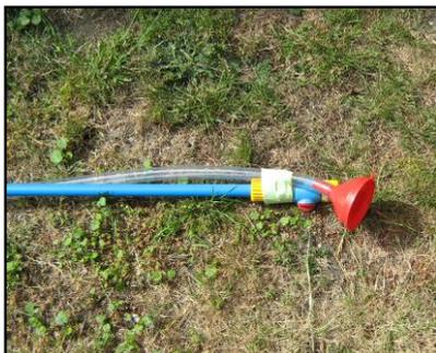
**4)** If you are unable to enter the tank, attach the funnel to a long pole that you can manoeuvre through the tank opening.
